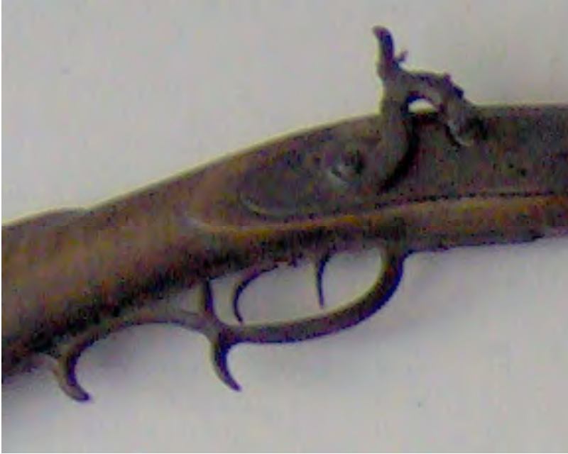
Close up view of double trigger mechanism made by William Edmundson Friend
